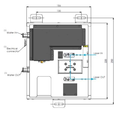
(1) Not included in ESUS product: cooling device and power supply unit for the pump diode
