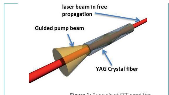
Figure 1: Principle of SCF amplifier
