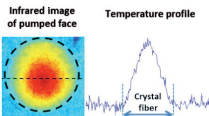
Figure 5: Thermography image of a pumped SCF module
